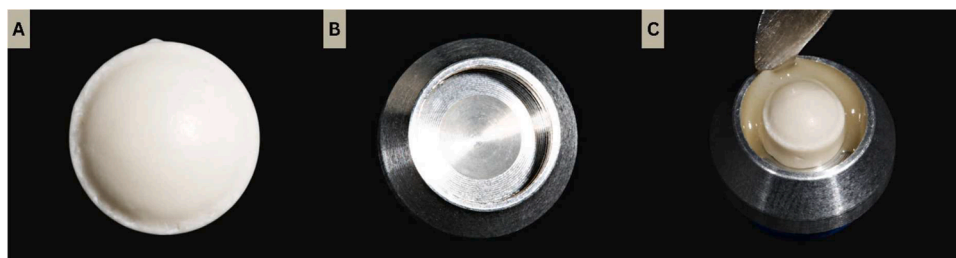
Fig. 5. A. Steatite antagonist. B. Metallic specimen holder for the embedding the antagonists and fixation in the chewing machine. C. Embedded steatite antagonist.
